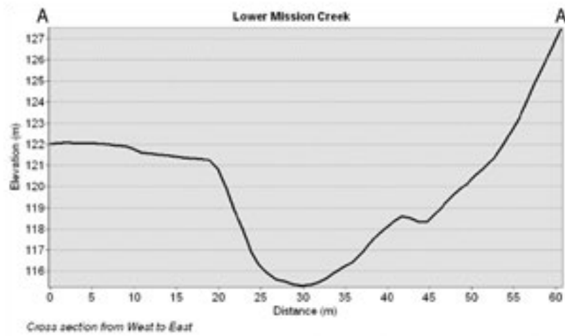
Figure 4.1.1. (a) Map of Lower Mission Creek survey reach showing the location of pools, groundwater springs, and impediments to fish passage. Note the lack of pool development upstream of Hwy 192. (b). The confluence of Mission Creek and Rattlesnake Creek is upstream of Hwy 192. Cross-section representing the channel geometry for this reach (A– A').
